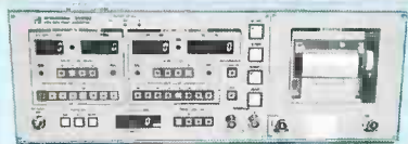
DROPOUT COUNTER used for measuring video dropouts.
